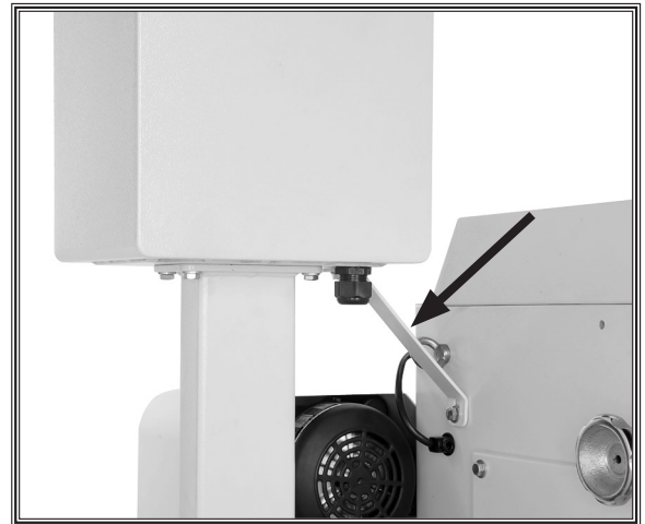
Figure 11. Control panel brace.
